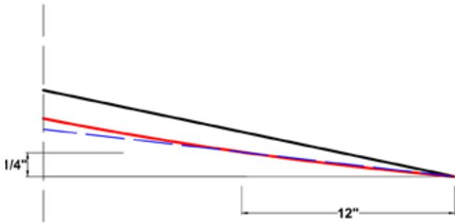
Figure 3: Increasing the code minimum 1/4 in 12 design slope to compensate for member total load deflection promotes free drainage and helps mitigate the potential for ponding by deflecting below a 1/4 in 12 surface.
