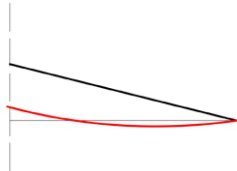
Figure 2: As the code-permitted L/120 or L/180 ratios are approached, the deflection curve extends below a horizontal datum to create a "bowl."
