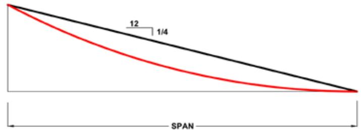
Figure 1: Wood members installed to a design slope of 1/4 in 12 often deflect from the initial dead load to create a "flat" area toward the low end.
